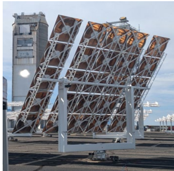
Actual Heliostat Image. This figure shows the heliostat alignment after using the RTO algorithm.
